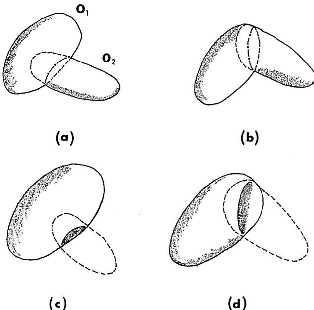
Fig. 2. Primitives can be combined through (a) generic penetration ( $O_1 \cup O_2$ ), resulting in a closed contour of concave discontinuity (---); (b) nongeneric penetration ( $O_1 \cup O_2$ ), resulting in an open contour of concave discontinuity; (c) generic subtraction ( $O_1 - O_2$ ), giving rise to a closed contour of convex discontinuity; and nongeneric subtraction (d), which will yield the same result as (c). Negative parts are indicated by dashed outlines.
