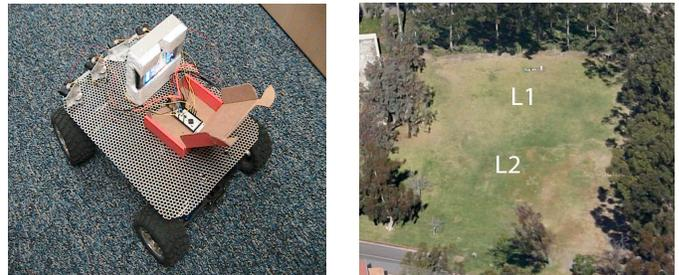
Fig. 1. Left - "Le CARL" robot constructed from the chassis of a R/C car. A base consisting of a sheet of perforated steel was mounted onto the chassis. Four infrared sensors, a phone holder, an Android smartphone, and the IOIO were mounted onto the base. Right - open grass field with both locations  $L_1$  and  $L_2$ , where the experiment was conducted.
