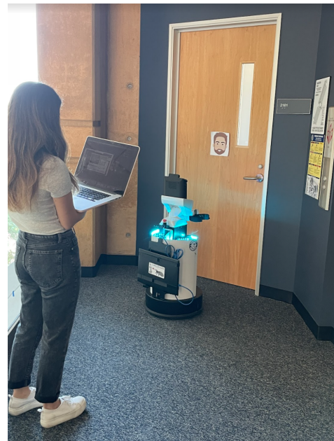
Fig. 3. HSR reaching a face location via telepresence operation. An experimenter, shown in the figure, was present to assist the remote participant if necessary.
