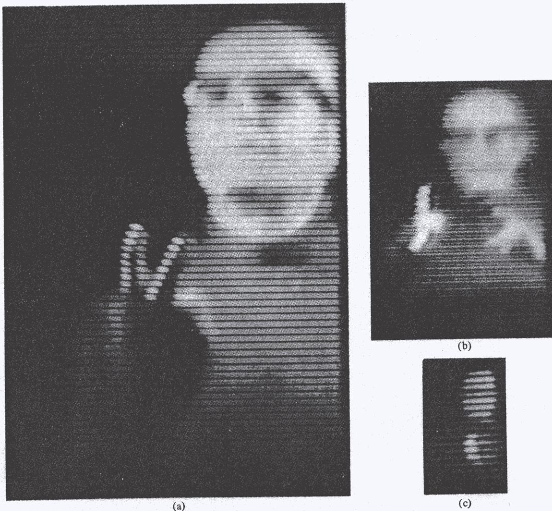
Fig. 2. Photographs of picture displays at three bandwidth conditions: (a) 86 300 Hz; (b) 21 000 Hz; (c) 4390 Hz. Exposure: 1/10 s, f/5.6, Polaroid ASA 3000 sheet film. The actual sizes of the three displays were 5.8 by 8.1 cm, 2.9 by 4.3 cm, and 1.31 by 1.96 cm. Because of quality losses in photography and in reproduction, the subjective quality of these photographs corresponds more nearly to the three lowest bandwidth conditions.
